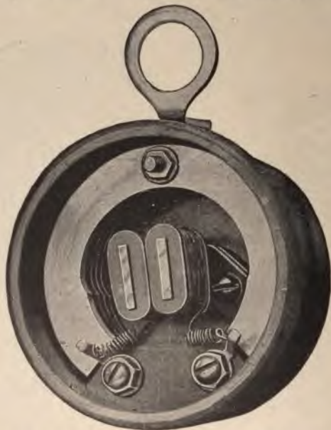
FIG. 75.—Interior view of a typical "watchcase" receiver.
